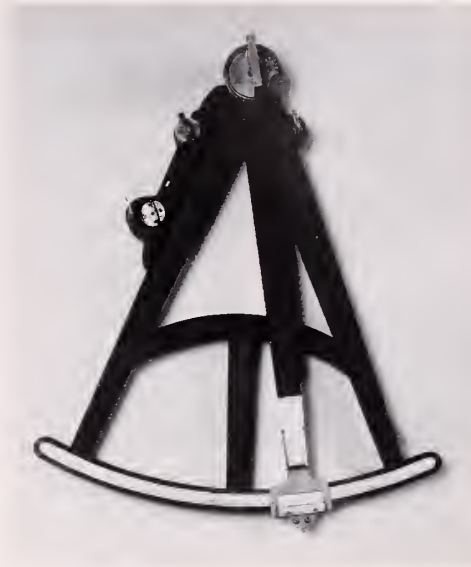
Octant (Hadley Quadrant), probably made in England, c. 1750. Wood, brass, and ivory; radius 17 1 / 8 " (43.5 cm). Collection of W. Horace Hepburn
